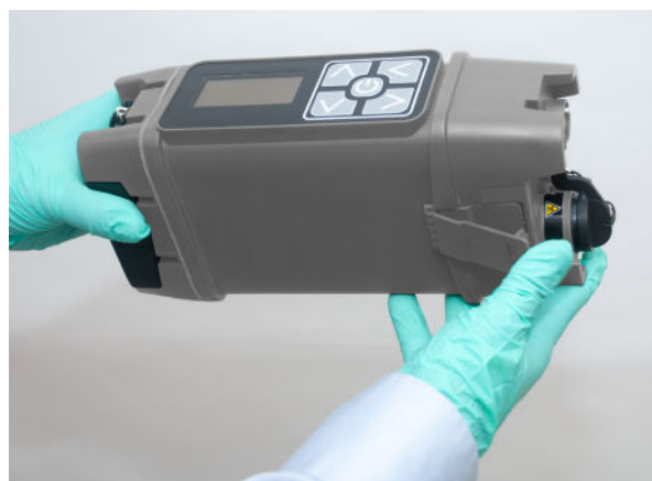
Clip front cover in place and power on the LCD 4 XID.
