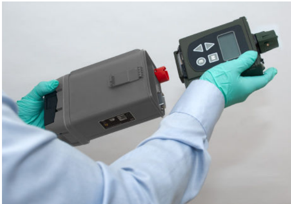
Slide LCD 4 into XID adapter.
