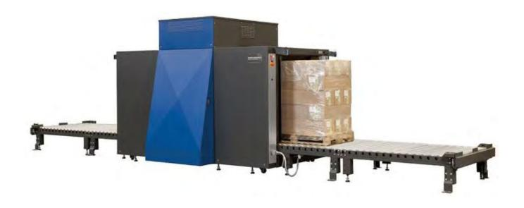
The *HI-SCAN 130130T-2is HD* for freight and euro pallets. It is equipped with two generators beaming in two directions (dual view). The second beam direction is displaced at 90° and thus facilitates reliable inspections of even tightly packed objects in only one process while shortening inspection times and increasing the effectiveness of the procedure.
